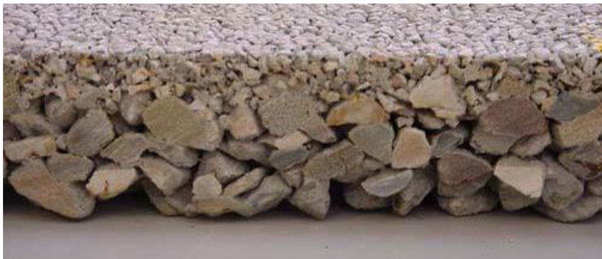
Rys. 33 Struktura nawierzchni dwuwarstwowej (Evaluation of U.S. and European Concrete Pavement Noise Reduction Methods, National Concrete Pavement Technology Center, 2006)
