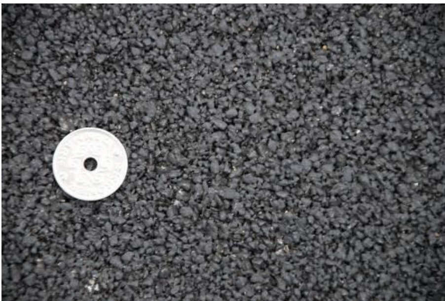
Rys. 24. Nawierzchnia jednowarstwowa (DVS-DRI Super Quiet Traffic International search for pavement providing 10 dB noise reduction, Danish Road Institute Report nr 178, 2009)
